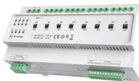
The TL55 is an AC-input, 8-channel switch actuator designed based on the DALI protocol. Each channel supports a maximum control current of 16A, making it suitable for on/off control of devices rated at 16A or lower.
